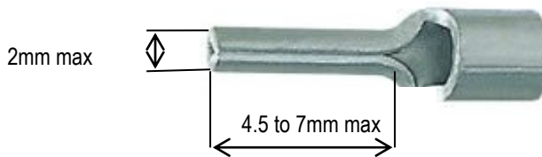
2-17 Lead Terminal for C22
